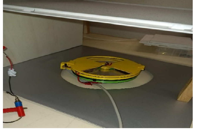
Fig. 7: 3D printed electric field mill with the parallel plate setup
