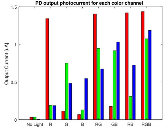
Fig. 2: The output photocurrent for each color channel at each one of the eight possible states and for an illuminance of 1943lux provided by a 4000K RGB LED. The first state is when no light was applied.
