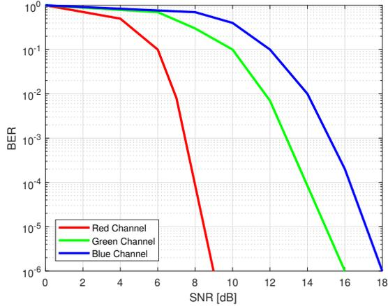
Fig. 7: Curves of BER versus SNR for the three channels of the photodiode.
