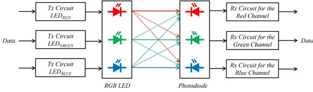
Fig. 1: The cross-channel interference among the three channel signals that are received by the photodiode. Note that a single RGB LED and a single RGB photodiode are used in this link.
