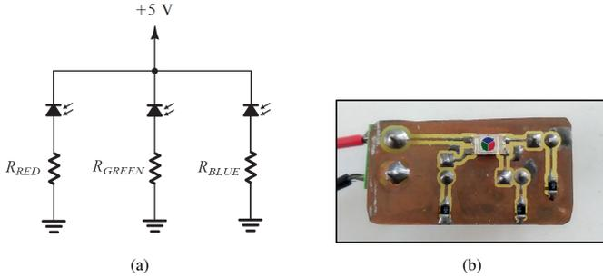
Fig. 6: (a) The receiver circuit using a triple photodiode topology with a common cathode. (b) The RGB photodiode receiver implementation.
