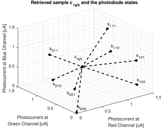
Fig. 3: Euclidean distance between the received color  $c_{rgb}$  and the eight different possible states.
