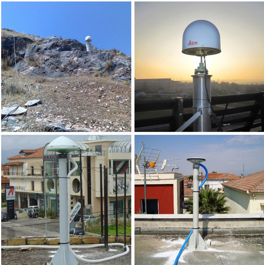
Fig. 2 Field photographs showing geodetic antennas used in this study: Station KLOK (top left), Station LARM (top right), Station KRDI (bottom left), Station STEF (bottom right)
