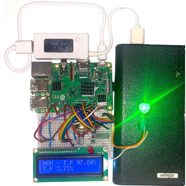
FIGURE 4. Microprocessor-based implementation of the proposed AF termination prediction system. The LCD display depicts the real-time soft-decision estimation of every prediction (AF or Non AF).
